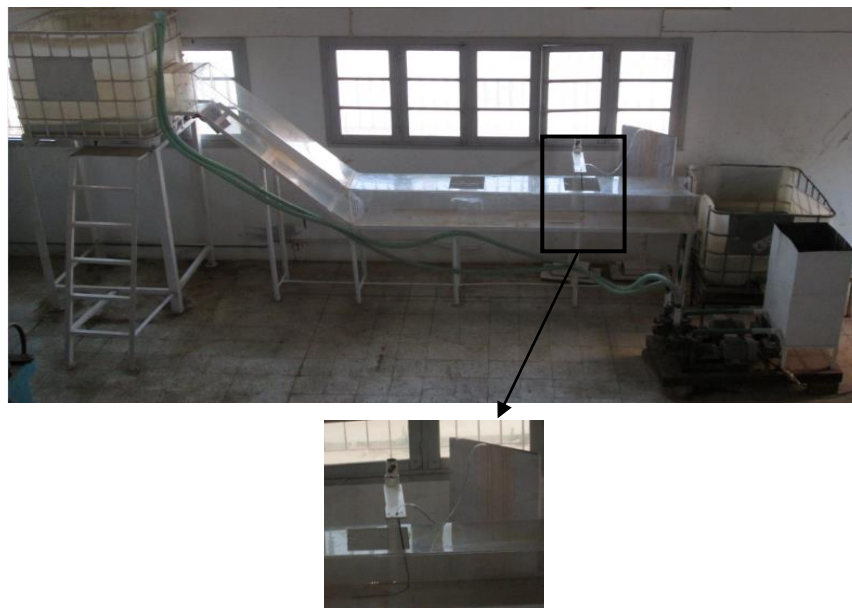
Fig. 32 Hydrodynamic test bench with Pitot tube
